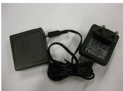
Balanced to non balanced converter box. For speakers with non balanced input only.
